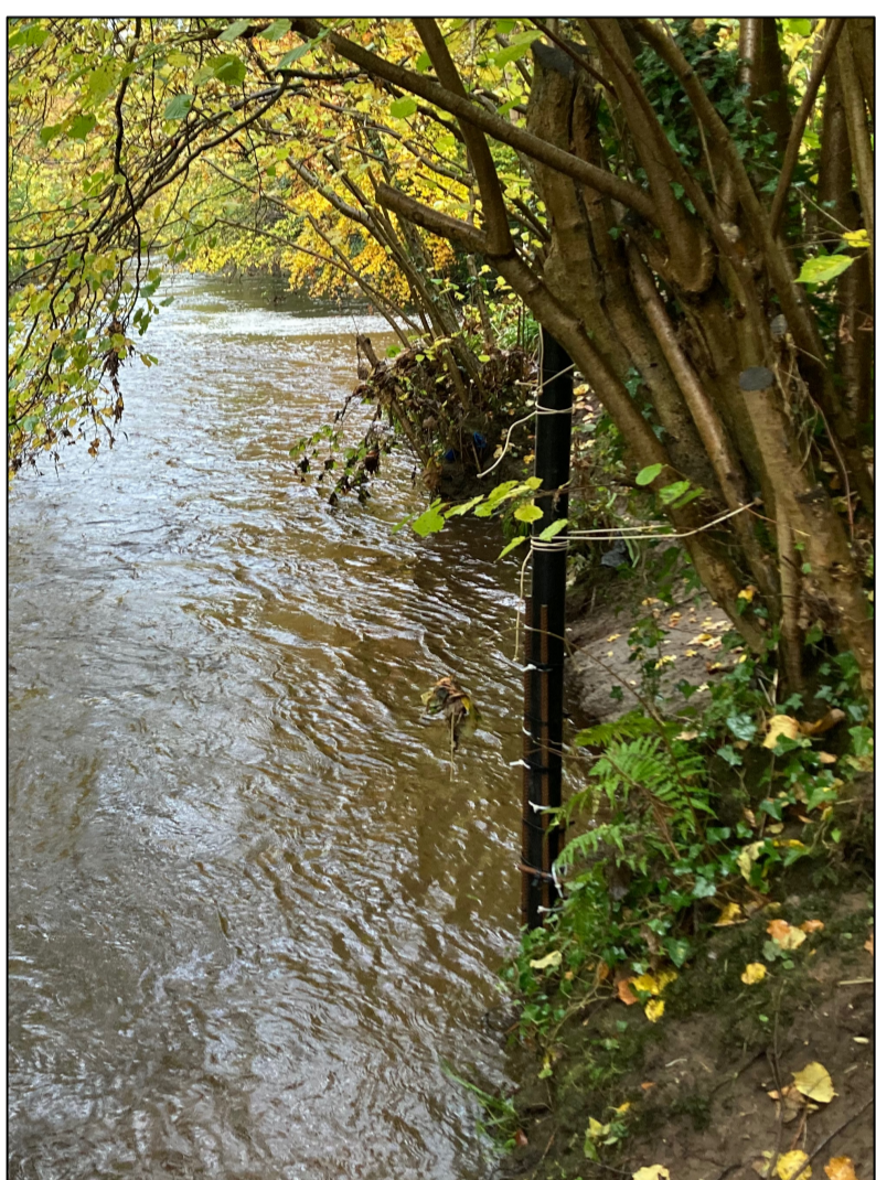
Figure 4: Stilling well, River North Esk.
